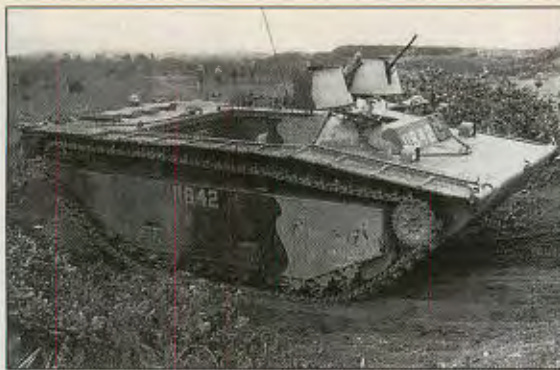
The LVT-2 amphibious vehicle transport, the "Grandfather" of the current amphibian assault vehicles, mounting an M1919A4 .30 caliber and a .50 Ma Deuce machine gun, on Iwo Jima during WWII.
